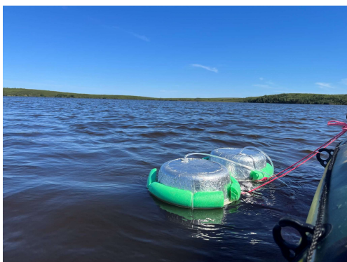
Floating chambers used to measure gas emissions from lakes
