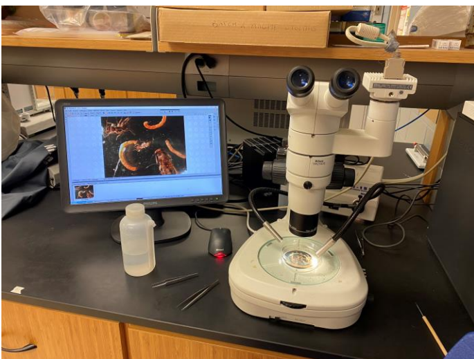
Photo (left): Dissecting microscope used to sort invertebrates by family. Photo by Mathew Mervyn.
